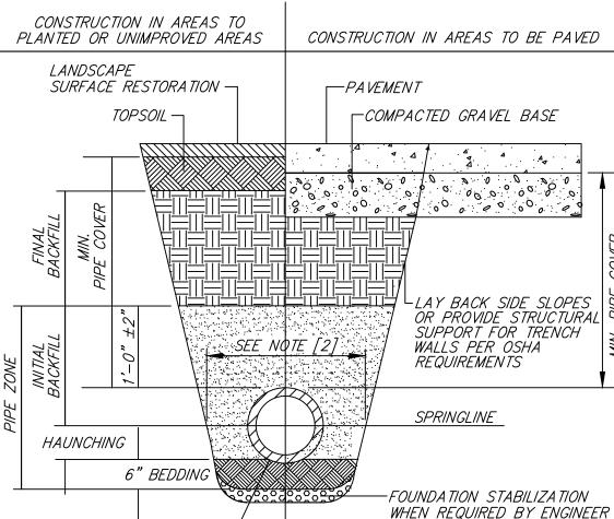
SHAPE BEDDING BY HAND -----TO FIT BOTTOM OF PIPE; INSTALL PIPE ON STABLE BEDDING WITH UNIFORM BEARING UNDER FULL LENGTH OF PIPE BARREL.
