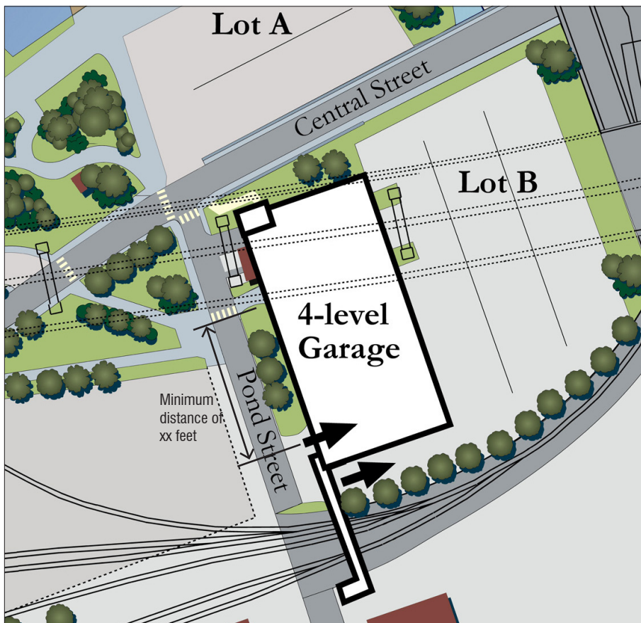
This graphic example represents a standard for the location of garage entrances and access.
