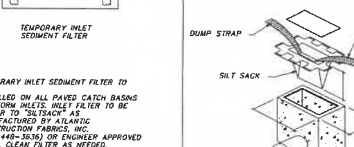
SILT SACK DETAIL NO SCALE
